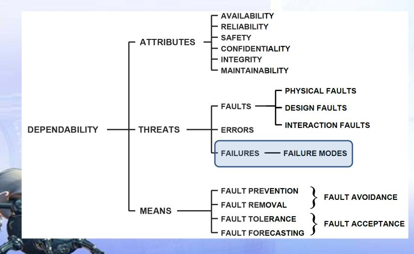
The way in which a system can fail are its failure modes, characterized by the severity and the symptoms of a failure.
